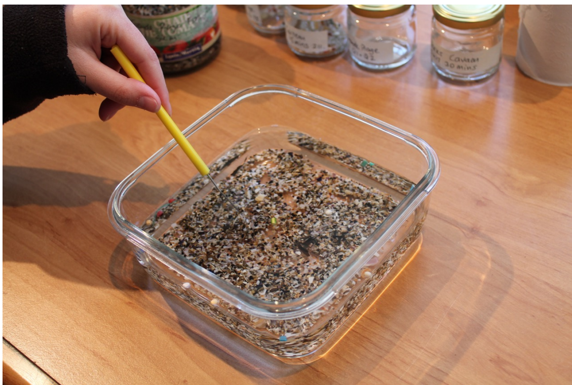
Figure 7: The 1 to 5mm items sieved from the sand being mixed with seawater
