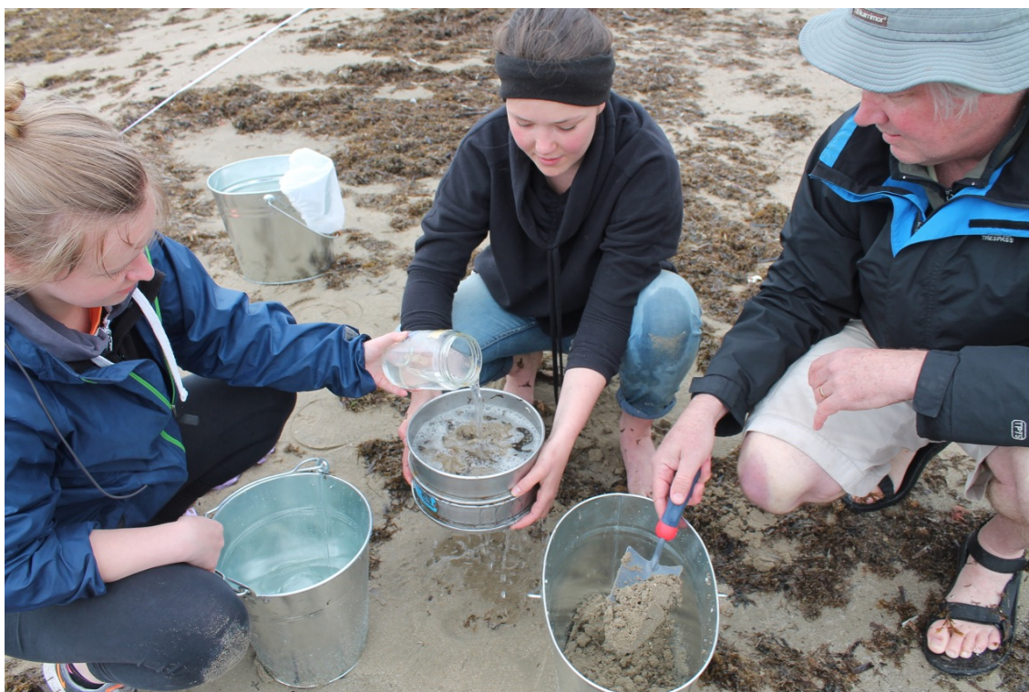
Figure 5: Sieving the sand through 5 and 1mm sieves – items between 1 and 5mm in size will accumulate on the surface of the bottom 1mm sieve
