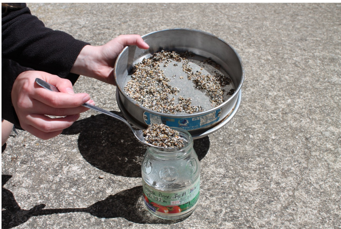
Figure 6: Collecting all the 1 to 5mm sized items from the surface of the 1mm sieve for subsequent separation of the microplastics from the other items
